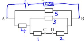
What resistance would be measured between terminals A and B? If a 6 V battery with an internal resistance of  $125\,\Omega$  is connected across terminals A and B, what current flows in the wire connecting terminals C and D?
