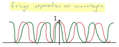
The narrow slits act like coherent sources, which means they have a constant phase difference between them. Light from those sources arrive at a particular point on the screen having travelled different distances. This is called path difference. Since the sources are coherent, the path difference at a particular point on the screen does not change.
