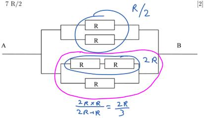
$$R_{+} = \frac{R_{2} \times 2R_{3}}{R/2 + 2R_{3}}$$
